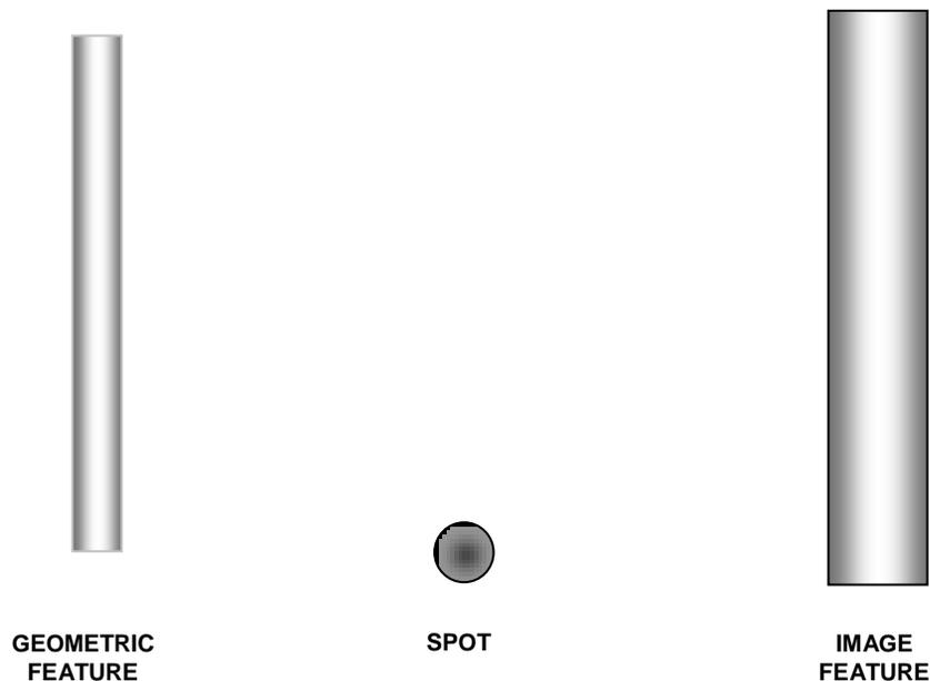
**FIGURE 7. GEOMETRIC FEATURE DIMENSIONS ARE INCREASED BY THE IMAGING SYSTEM SPOT DIAMETER**
