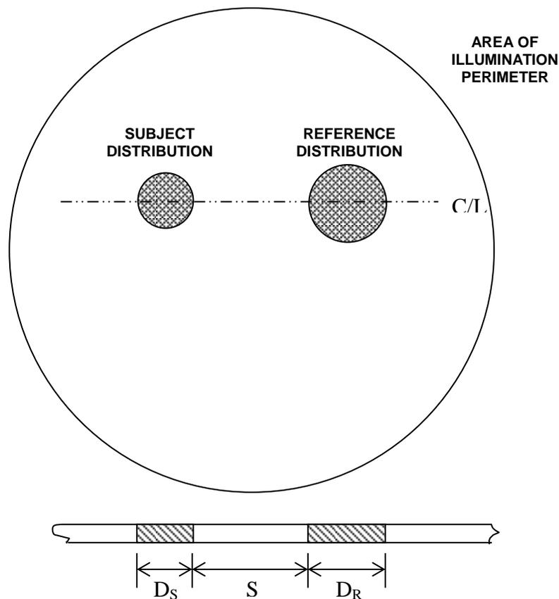
FIGURE 5. RIF OBJECT PLANE CONFIGURATION: PLAN AND FRONT ELEVATION VIEWS
