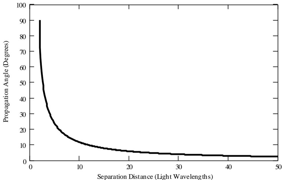
**FIGURE 4. OBJECT SIDE PROPAGATION ANGLE  $\theta$  AS A FUNCTION OF THE SEPARATION DISTANCE  $\Delta$  BETWEEN TWO POINTS IN THE OBJECT**
