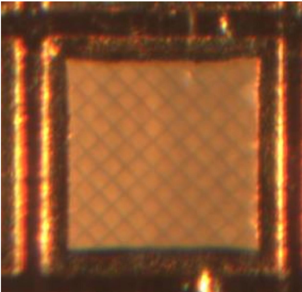
**FIGURE 11. QUANTIFOIL S7/2 MICROMACHINED SQUARE MESH HOLEY CARBON GRID**
